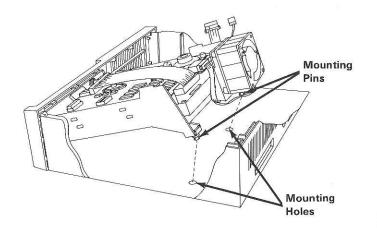
16 Position the diskette drive and fan power cables as shown below.
