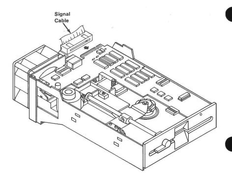
Place the signal cable on the top of the diskette drive. Place the diskette drive and fan power cables underneath and out the side of the diskette drive unit.
