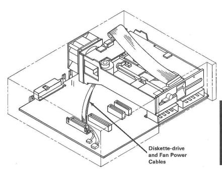
Position the power board so that its system connector and two pin connectors are directly above its system slot and two pin plug. Press it firmly into place. Be sure that the rear of the power board goes into the rear guide.
