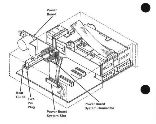
18 Plug the fan and the diskette drive power cables into their connectors.
