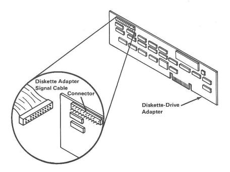
20 Position the diskette drive adapter so that its system connector is directly above its system slot, press it firmly into place. Be sure that the rear of the diskette drive adapter goes into the rear guide.
