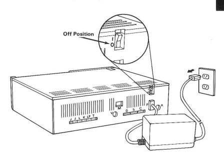
Warning: After turning your IBM PCjr power off, allow 5 minutes for cooling to take place before removing the cover.
