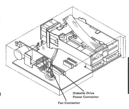
Plug the diskette drive signal cable into the connector on the diskette drive adapter. Be sure to align the pins and holes correctly.
