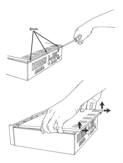
Remove diskette face plate by pushing on it from inside the IBM PCjr. It will snap out.
