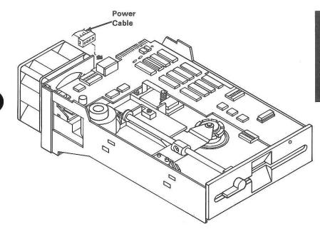
12 Unpack the signal cable from its box. Plug the folded end of the signal cable into its connector on the diskette drive. Be sure to align the guide correctly.
