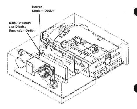
Replace the top cover by placing it on the IBM PCjr. Slide it forward until the top cover and front of the IBM PCjr fit together. Press down on the rear of the top cover until it snaps into place.
