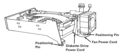
Place the diskette drive unit into the IBM PCjr. Make sure the front guide goes into the front panel slot.
